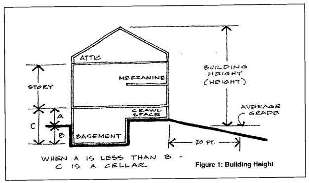
**BUILDING HEIGHT:** The vertical distance of a building measured from the average elevation to the finished grade within twenty feet of the structure to the highest point in the roof. (see Figure 1)
